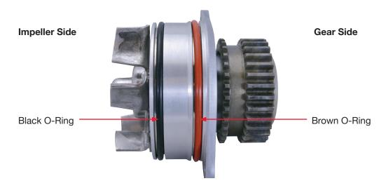
Install the smaller black O-ring in the groove towards the "IMPELLER SIDE" of water pump as shown. Install the larger brown O-ring in the groove towards the "GEAR SIDE" of the water pump as shown.
